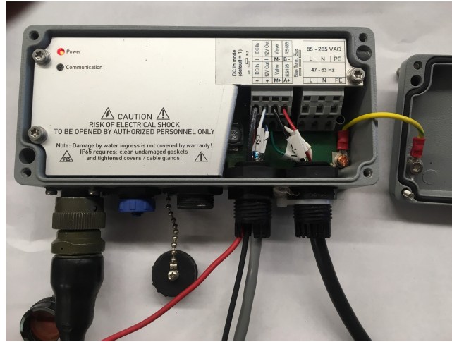
Figure 2.1: picture of the connecting capabilities inside the Con::nect Box
