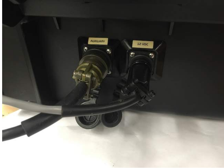
Figure 2.6: External plugs for the 2-pin and 6-pin cables
