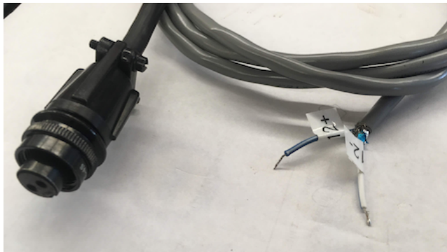
Figure 2.3: 2-pin cable to provide 12V DC power to the MUX, with the blue wire as '+' and the white wire as '-'
