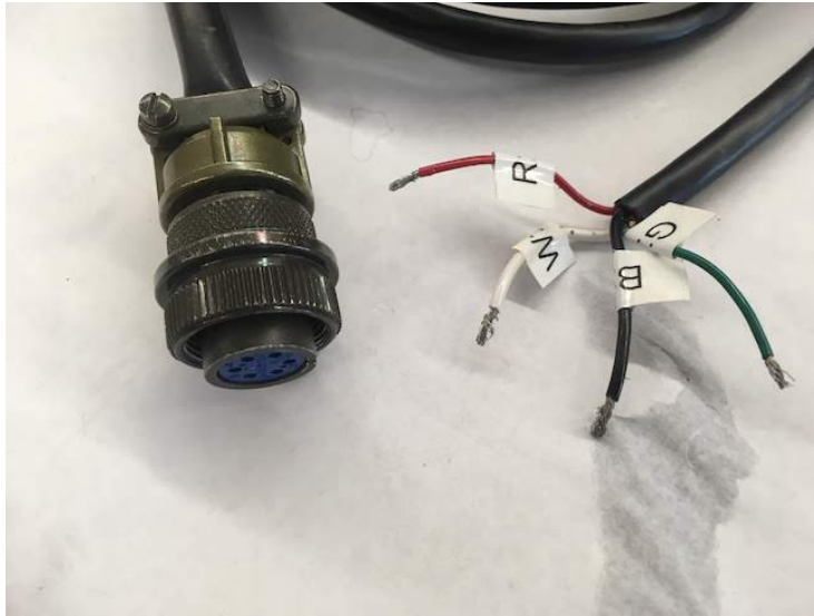
Figure 2.5: 6-pin cable to trigger a sampling sequence to the MUX, using the black (M-) and green (M+) wires, and, to communicate between the MUX and the spectrolyser using the white (A+) and the red (B-) wires through the RS485 protocol
