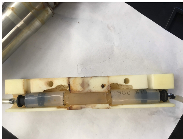
Figure 6.2: Flow through cuvette installed in its cuvette holder
