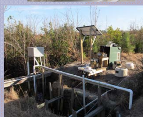
Fig. 6. Continuous monitoring station and automated sampler located at the outlet of D3
